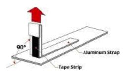
Peel Tested @ 300mm/min All data shown in N/cm
