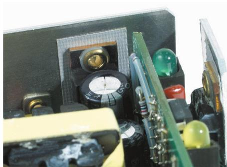
Sil-Pad® 400 is a composite of silicone rubber and fiberglass. The material is flame retardant and is specially formulated for use as a thermally conductive insulator. The primary use for Sil-Pad® 400 is to electrically isolate power sources from heat sinks.
