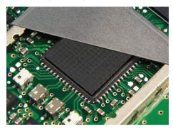
Gap Pad® EMI 1.0 is a highly conformable, combination gap filling material offering both thermal conductivity performance and Electromagnetic Energy absorption (cavity resonances and/or cross-talk causing Electromagnetic Interference) at frequencies of 1GHz and higher.
