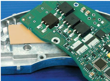
Gap Pad® A3000 is a thermally conductive, filled-polymer laminate, supplied on a reinforcing mesh for added electrical isolation, easy material handling and enhanced puncture, shear and tear resistance. Gap Pad® A3000 has a reinforcement layer on the dark gold side of the material that assists in burn-in and rework processes while the light gold and soft side of the material allows for added compliance.
