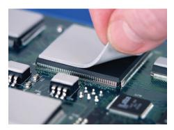
Gap Pad® 2000S40 is recommended for low-stress applications that require a mid to high thermally conductive interface material. The highly conformable nature of the material allows the pad to fill in air voids and air gaps between PC boards and heat sinks or metal chassis with stepped topography, rough surfaces and high stack-up tolerances.
