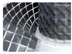
Gap Pad® 1500R has the same highly conformable, low-modulus polymer as the standard Gap Pad® 1500. The fiberglass reinforcement allows for easy material handling and enhances puncture, shear and tear resistance. The natural tack on both sides of the material allows for good compliance to mating surfaces of components, further reducing thermal resistance.
