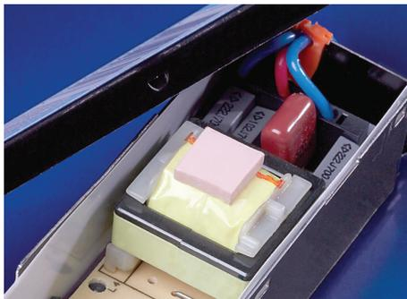
Gap Pad® 1450 is a highly compliant Gap Pad® material that is ideal for fragile component leads. The material includes a PEN film, which facilitates rework and improves puncture resistance and handling characteristics. The tacky side of Gap Pad® 1450 maintains a conformable, yet elastic nature that provides excellent interfacing and wet-out characteristics, even to surfaces with high roughness or uneven topography.
