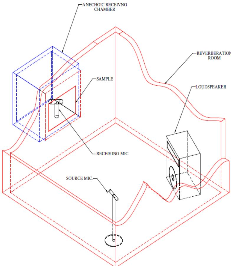
The test procedures for the STL test conformed to that specified by SAE recommended practice for the “Laboratory Measurement of Airborne Sound Barrier Performance of Automotive Materials and Assemblies” – SAE J1400 August, 2010.
